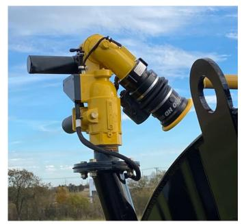
The HOLT Spray King is equipped with a Nitro HD® monitor and joystick controller. The joystick provides basic directional movement of the monitor and actuation of the nozzle.
