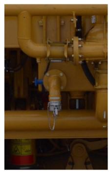
At left, remove fitting at the front of the tank to drain the tank and the pump.
