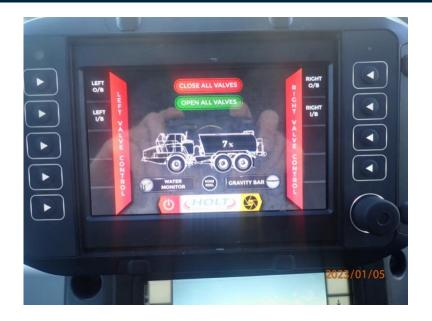
After starting the vehicle there are two ways to engage the rear spray heads.
