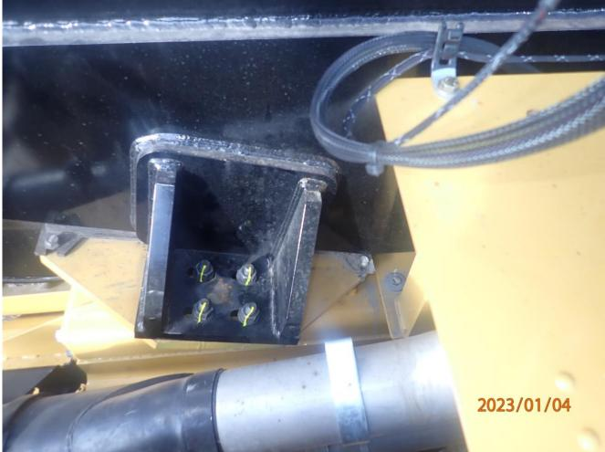
4. Remove 8 bolts from front mounts – shown here is one mount on one side. Remove mounts from both sides.
