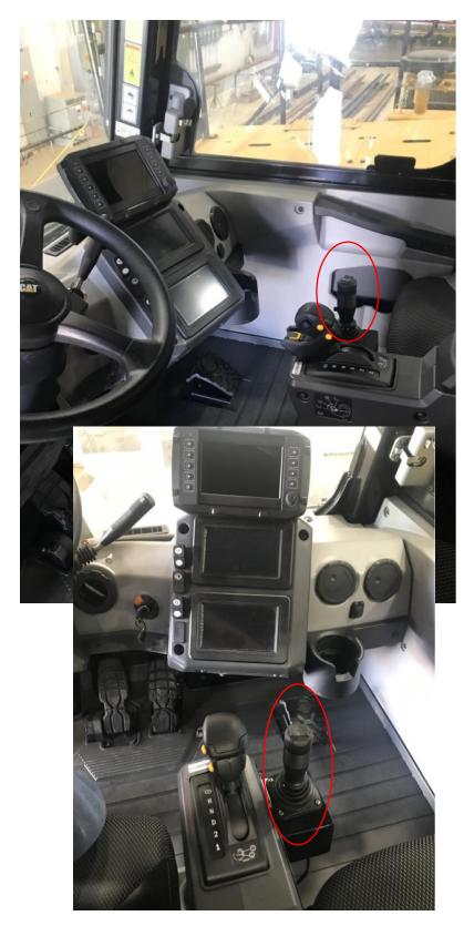
Use the joystick to control the direction of the water spray.
