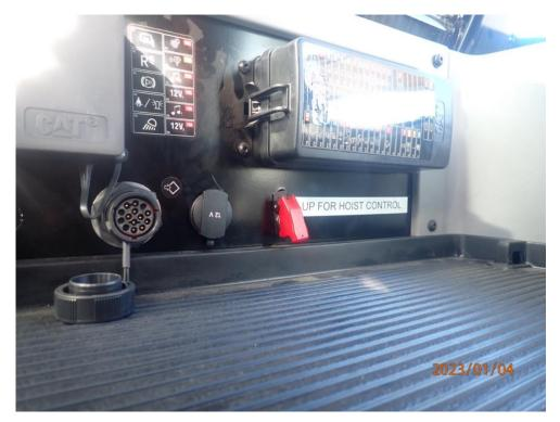
SECOND GENERATION: Inside cab, behind driver seat, above and to the left of the fuse box, there is a safety lock key control. Turn the key on transfer hydraulic engagement from the screen back to the hoist switch on the shift selector.
