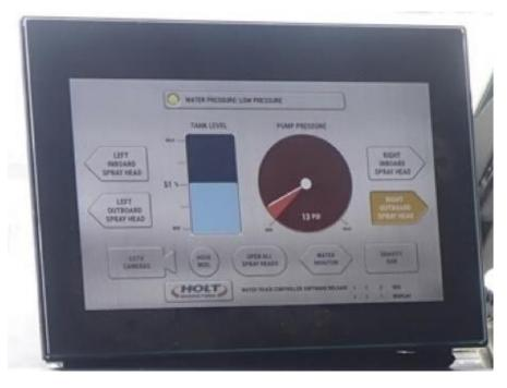
Touch the HOSE REEL circle, then touch the WATER MONITOR bar. The WATER MONITOR bar will illuminate, and the spray symbol on the truck diagram will indicate engagement.
