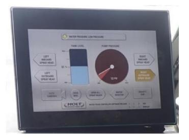
When using the gravity bar, it is not necessary to operate at higher RPM as the water is released only with gravity and not under pressure.
