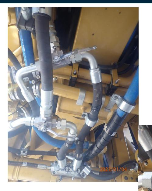
5. Under center of machine there are two manual directional ball valves. Remove safety tie strap and open both valves. This will allow hydraulic oil to be diverted from water tank back to cylinders.
