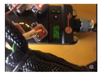
Missing wire seals. In connector CON17 main power into IFM controller.
