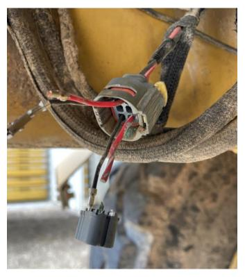
Pin to wire connection failure.
