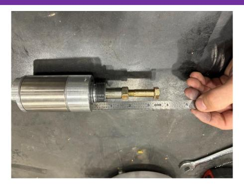
Using 1¼" wrench install actuator to spray head housing.
