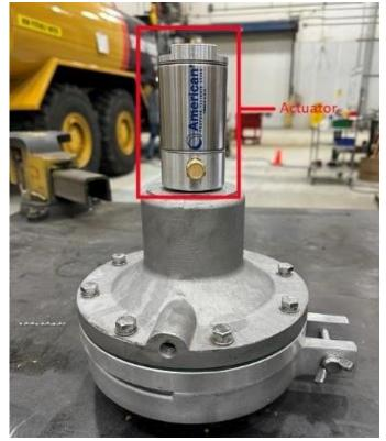
Measure actuator from the base to the end of the adjuster bolt.
